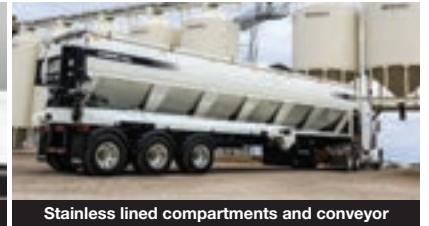
Stainless lined compartments and conveyor
