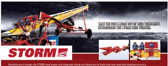
Electronic controls feature touch screen input and pre-programmed recipes. The metering conveyor accurately measures seed flow and automatically adjusts the peristaltic pumps to match treatment flow for optimal coverage, the first seed to the last. The STORM is suitable for a wide variety of seed types including wheat, barley, oats, peas and lentils.
